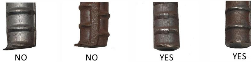
Acceptable and Non-Acceptable Rebar End Preparation
